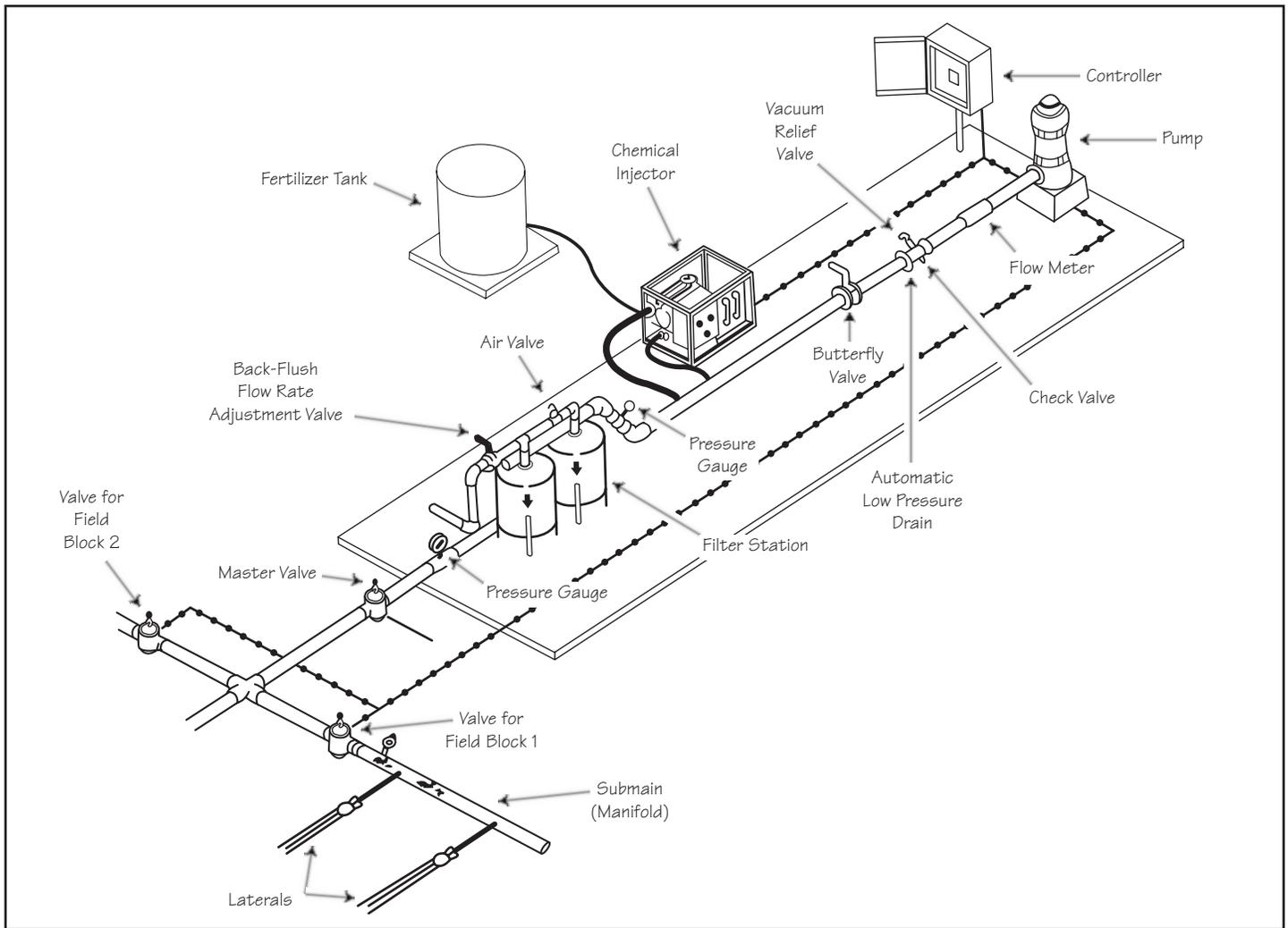
Figure 1. Typical layout of the irrigation system.
