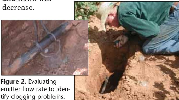
**Figure 2.** Evaluating emitter flow rate to identify clogging problems.
