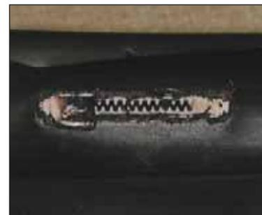
**Figure 4.** An emitter clogged by manganese oxides.
