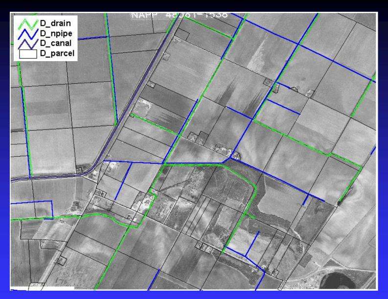
Drainage, pipe, and canal systems also drawn into ArcView using DOQQ as a reference.
