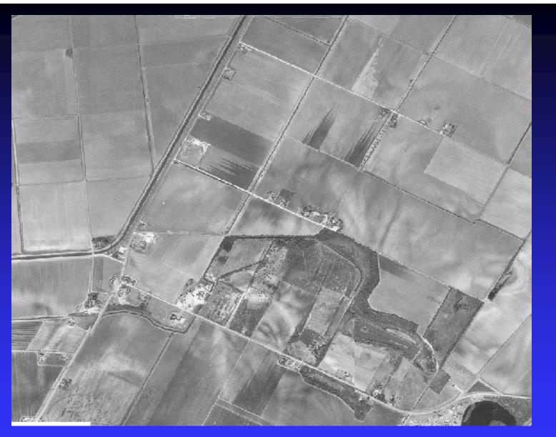
Inserting DOQQ - Digital Orthophoto Quarter Quadrangle These are infrared satellite images that can aid in drawing land parcels.
