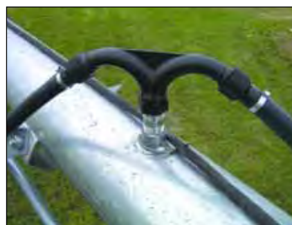
Figure 12.a. A double barb gooseneck.
