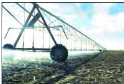
Figure 6. Drops with LESA applicators.
