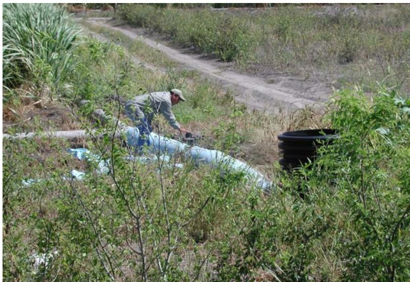
**Figure 8. Recording flows with in-line saddle propeller meter.**
