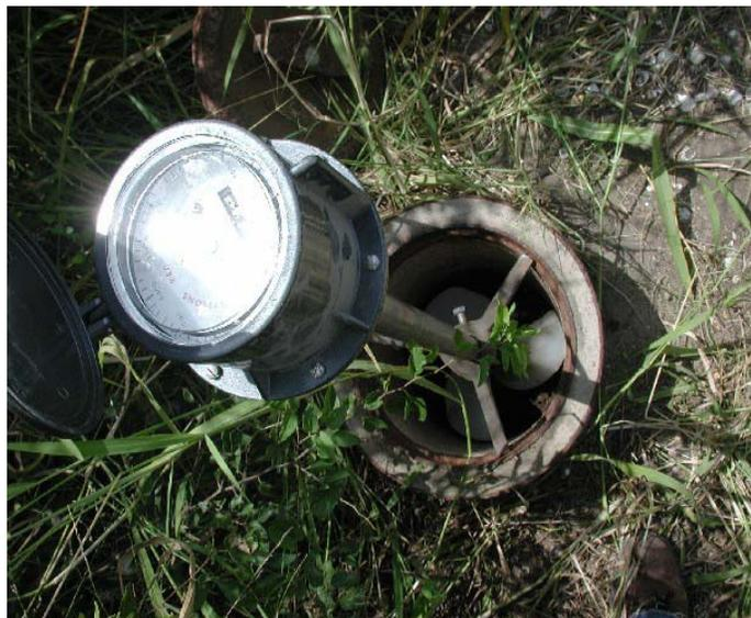
**Figure 6. Vertical flow meter ready to measure farm outlet.**
