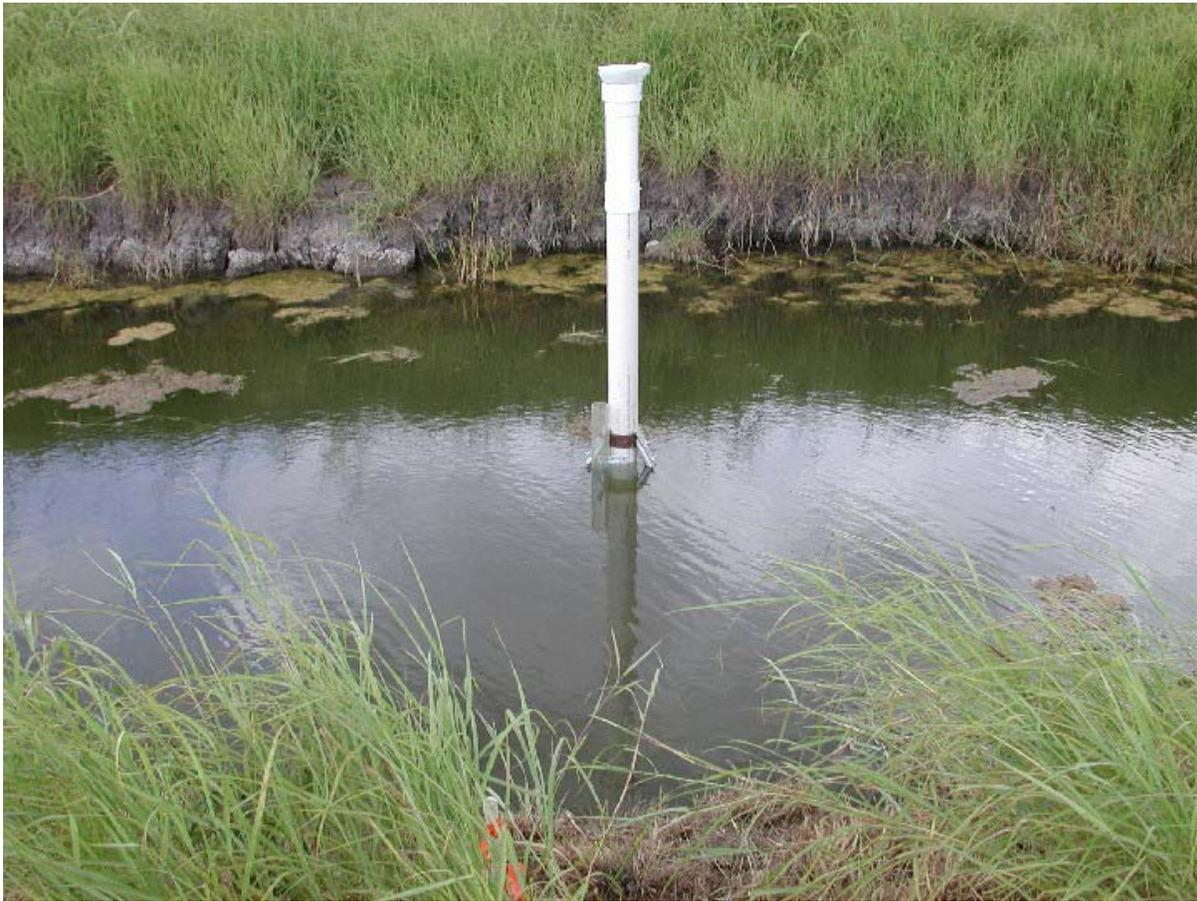
**Figure 2. Continuous-stage level recorders on canal 55.**
