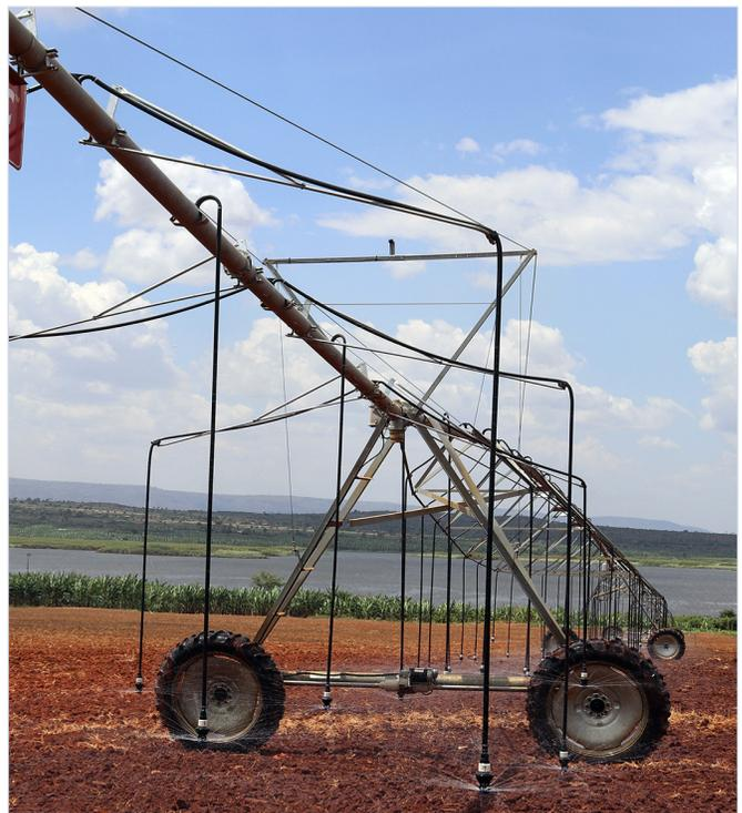
Figure 16. An example of a simple suspension boom-back design.
