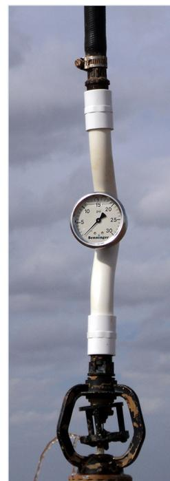
Figure 13. Pressure gauge drip.
