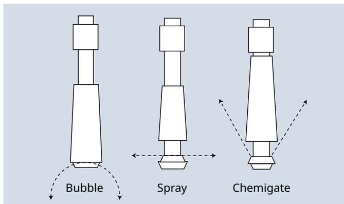
Figure 10. Original multi-functional LEPA head.
