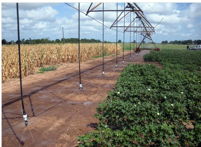
Figure 7. Close drop spacing with LESA water applicators.
