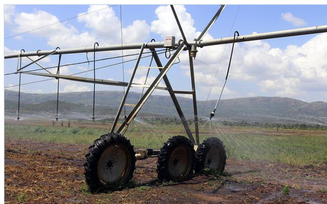
Figure 15. Wheels and pivot components catching and concentrating irrigation water at the towers/wheels.
