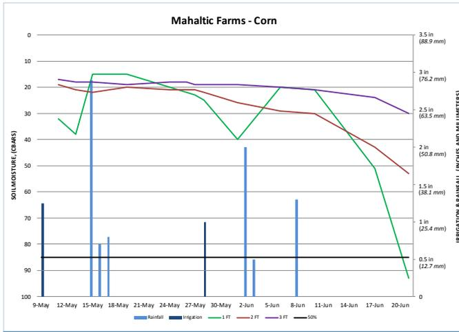
**Figure 17. Soil moisture measurements in a corn field on a heavy clay soil, with sensors located at 1, 2, and 3 feet (30, 60, and 90 cm). Soil moisture levels should not fall below a reading of 85 for this particular soil.**
