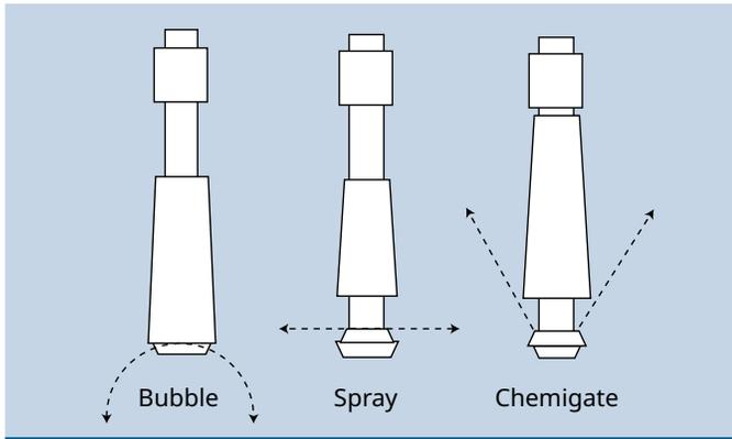
**Figure 10. Original multi-functional LEPA head.**
