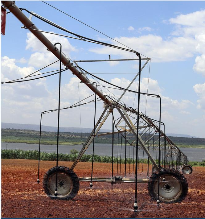
**Figure 16.** An example of a simple suspension boom-back design.
